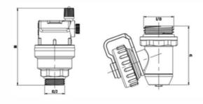
The Tio componentry included an automatic air vent with a 1/2 inch inlet and a drain/fill valve with a 1/2 inch inlet.
